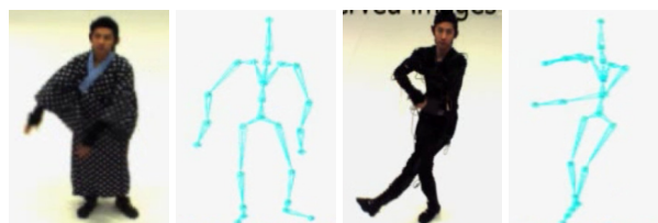
Figure 9. Incorrect pose estimation results by detection with GPDM (i.e., M3). Left: dance (different arm directions), Right: exercise (upside down arms).
